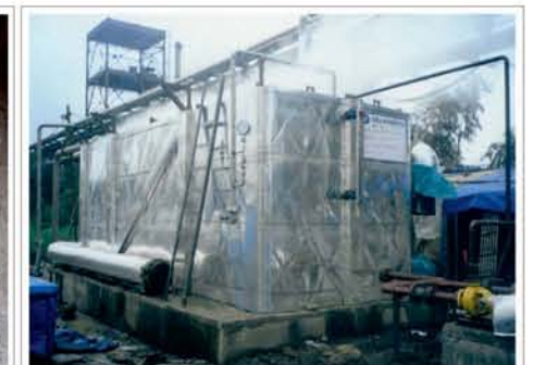
20 TONS / HR , 30 BAR Steam Bath Vaporizer
