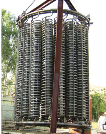
Coils inside the UHE 200 heat exchanger.
